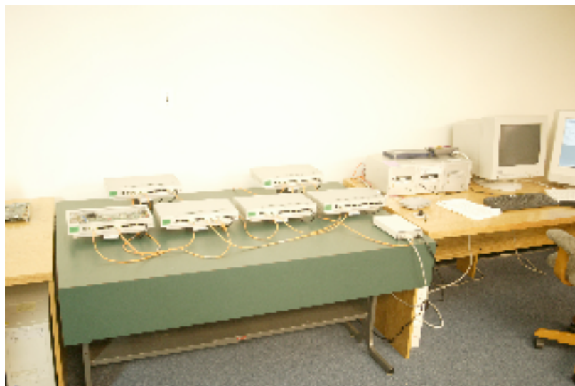
The “train set Mk2” - a prototype 155 Mb/sec switched fiber access network
